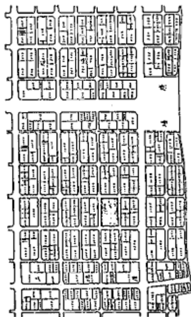
Pattern after pooling/readjustment- including new street layout, parkland, and sites for city expansion Kaohsiung City, Taiwan
