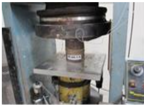
Figure: 4: Setup of compression test of bamboo
