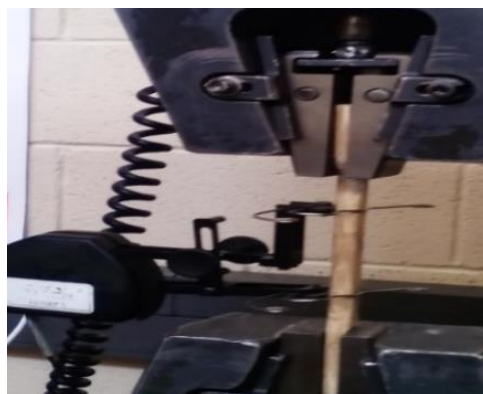
Figure 5: Setup of tensile test parallel to grain of bamboo
