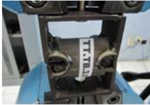
Figure 6: Setup of tensile test perpendicular to grain test of bamboo
