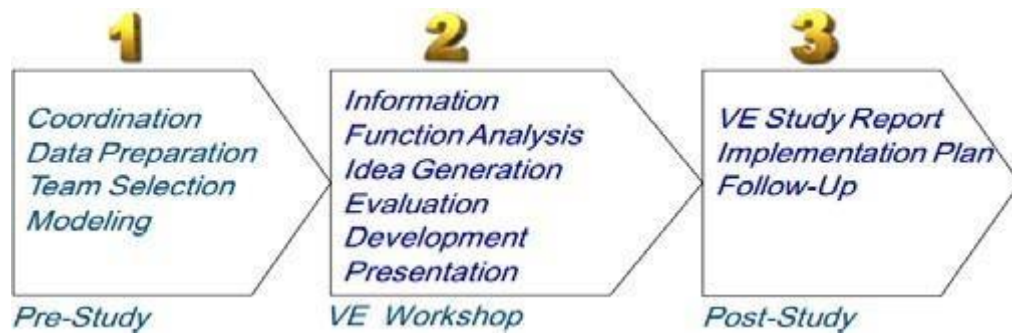
Figure 2: Value engineering flow process diagram - Source: (John and Paul 2007)
